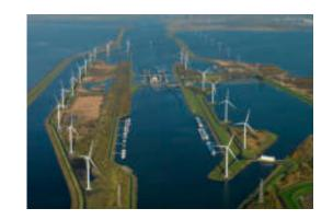
The onshore wind farm Kreekraksluis is located on and near the Kreekrak locks on the Scheldt-Rhine Canal in the Zeeland municipality of Reimerswaal in the Netherlands. The wind farm has a capacity of 40 MW from 16 Nordex 2.5 MW turbines.
